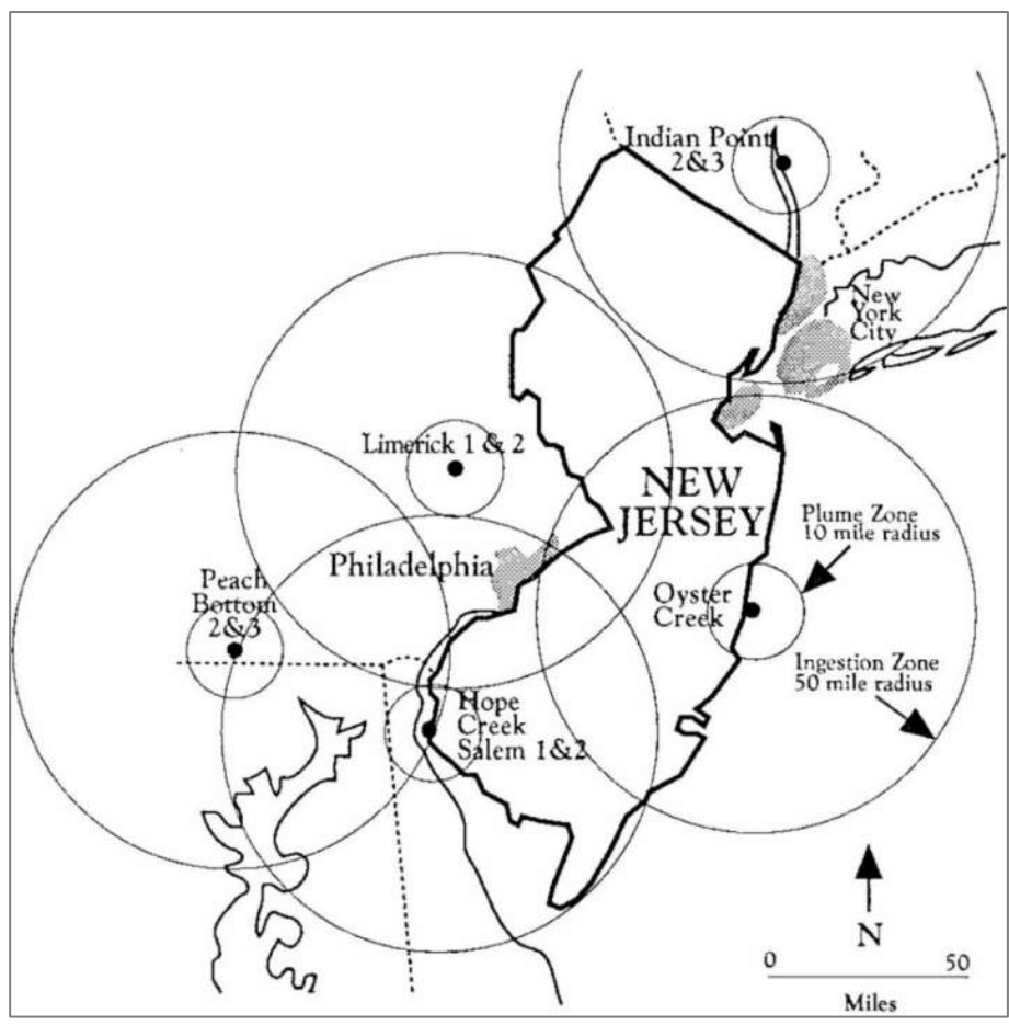
Figure 4.3.12-2 50 Mile Ingestion Pathway Zone Map for All Nuclear Power Plants Affecting New Jersey (NJOEM, 2012)
